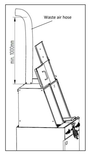
You can adjust the exhaust air flow at the throttles as needed for the length of the waste air hose.
